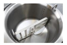
Uniform heating Food is evenly heated via the base and the side of the well of the pan at temperature 121 °C, maximum pressure 1.2 bar. Heat up 100 litres in 26 minutes.
