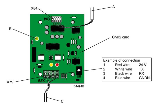
7 Mount the grommet in the hole Ø 16 on the top of the machine. Pass the wirenetwork cable C (4 x 0.22 mm²) in this grommet.
