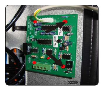
5 Connect the plug of Network cable A to terminal X84 of the CMIS Machine Interface.
