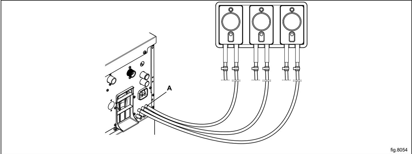
When all hoses has been connected, use cable ties to strap the hoses to the connections to make sure they are tight.
