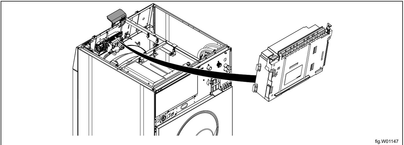
Strap the cable at suitable positions. The cable must not be in contact with the drum.
