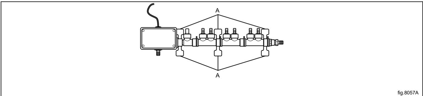
Connect the outlet tubes to the Flush manifold connections (B).
