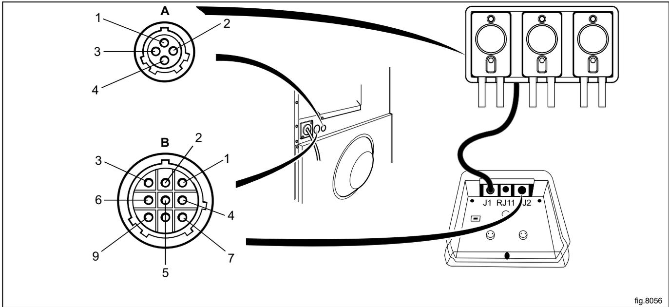
If the machine IS NOT prepared for external dosing systems from factory the cable from the J2 port on the EDS controller shall be connected to the RS232 port on one of the I/O modules in the machine. Follow the instruction for your type of machine.
