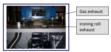
By law the exhaust outlet must be completely separated from the gas outlet to prevent the risk of fire.
