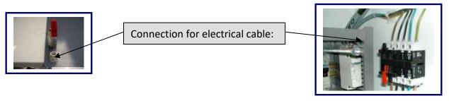
When the connection cable is connected, the main switch can be moved to position "1" and the direction of movement of the motors must be checked (to prevent damage).
