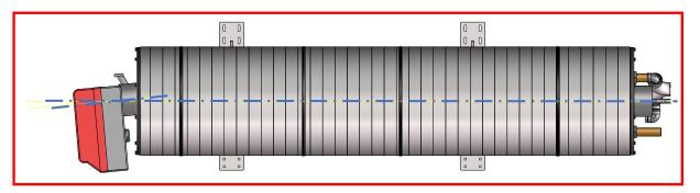
On startup of the machine on location, burner settings have to be adjusted by an qualified or certified technician and be inspected on standards in the concerned region. Before starting the burner, it is necessary to read the enclosed manual of the burner and the gas valve. Burner settings also have to be adjusted every 12 months for optimal burning and efficiency, also by an qualified or certified technician.
