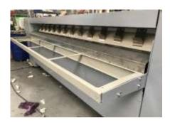
Dismantle the protective plate at the back.
