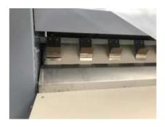
Allow the machine to warm up (adjust the temperature setting to 175°) and press start and at the same time press against the finger guard so that the bed closes and the roll does not turn. Loosen the tensioning screws and adjust the distance between the bed and bench so that they are 2 mm apart. Then tighten the tensioning screws again.
