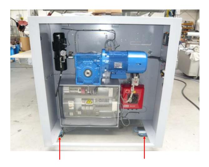
To place the rollers under the machine, the machine can be lifted with a hydraulic jack on these 4 supports.
