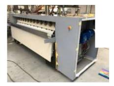
Undo bolts and rotate bench 90° so that you can screw the same bolt back in and place the bench flat (spirit level). Then tighten both bolts well.
