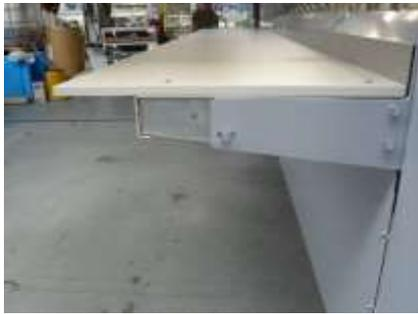
Tensioning screws at the bottom of the bench
