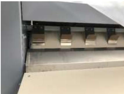
Allow the machine to warm up (adjust the temperature setting to 175°) and press start and at the same time press against the finger guard so that the bed closes and the roll does not turn. Loosen the tensioning screws and adjust the distance between the bed and bench so that they are 2 mm apart. Then tighten the tensioning screws again.
