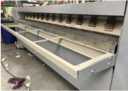
Dismantle the protective plate at the back.
