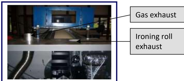
By law the exhaust outlet must be completely separated from the gas outlet to prevent the risk of fire.
