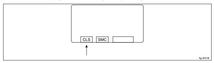
Press SMC to select a wash program from the smart card. (A smart card must be inserted in the program control unit).
