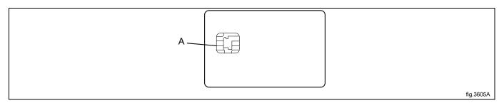
The smart card is capable of storing 10 to 15 wash programs of normal size. If the wash programs are mostly small ones, more of them can be stored, whereas larger wash programs will reduce the number which can be held by the smart card. Smart cards of this type can be used to:
