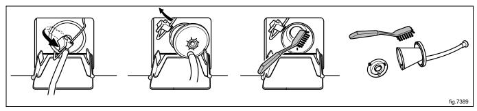
When remounting, place the cut on the filter part downwards when inserting it. Make sure the connections are tight.
