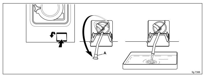
Pull the clamp upwards and pull out the filter parts. Clean the filter parts and the pump housing with for example a small brush.
