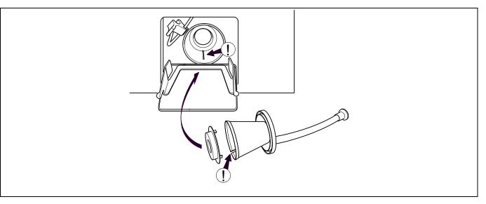
At regular basis, check the drain connection, joints in the drain pipe etc and remove any lint and dust. Clean with for example a small brush. When remounting, make sure the connections are tight.
