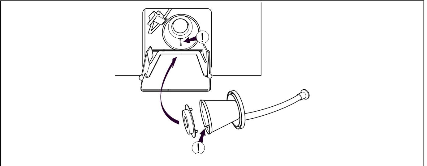
At regular basis, check the drain connection, joints in the drain pipe etc and remove any lint and dust. Clean with for example a small brush. When remounting, make sure the connections are tight.
