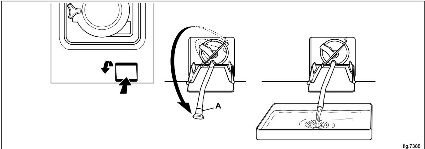
Pull the clamp upwards and pull out the filter parts. Clean the filter parts and the pump housing with for example a small brush.
