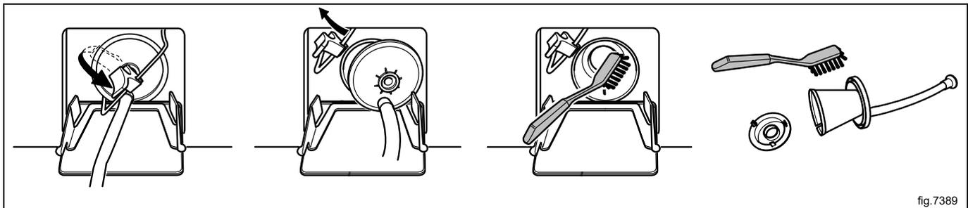
When remounting, place the cut on the filter part downwards when inserting it. Make sure the connections are tight.
