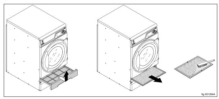
When the second lint filter has been cleaned, insert the second lint filter and the filter drawer.
