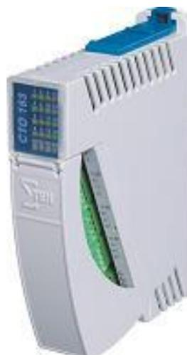
20 LED's are on the CDI163. The LED's 1-16 indicate if the corresponding input is high (LED on) or low (LED off). The lowest row of LED's indicates if the power supply of 24 Volts DC per group of 4 inputs is present. When the power supply is OK, the LED will light, otherwise, the LED will stay off.
