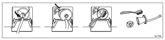
When remounting, place the cut on the filter part downwards when inserting it. Make sure the connections are tight.
