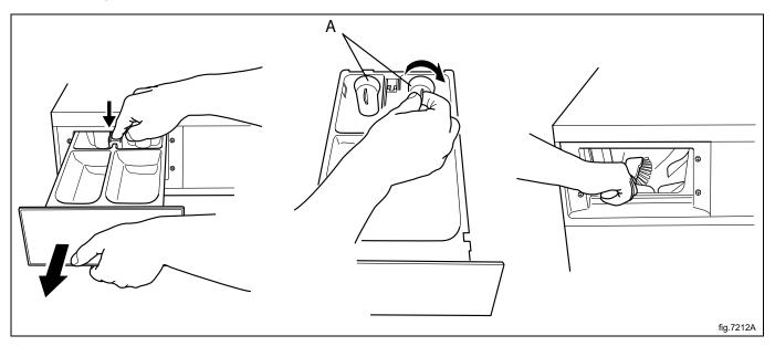
Use a screwdriver or a similar tool to press against the inner walls on the spraying plate to clean from limescale. Press carefully and not too hard since pressing too hard might damage the spraying plate.
