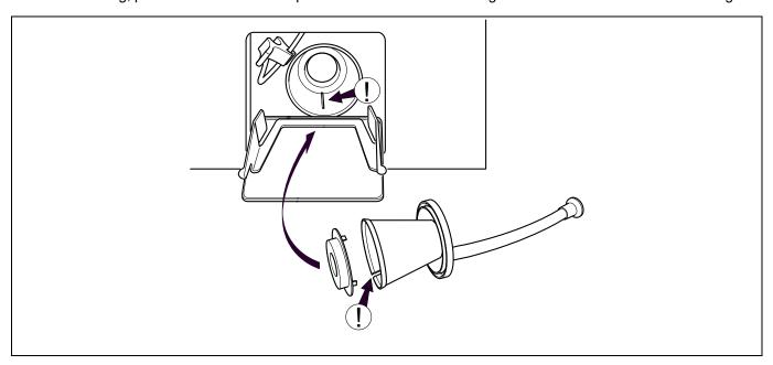
At regular basis, check the drain connection, joints in the drain pipe etc and remove any lint and dust. Clean with for example a small brush. When remounting, make sure the connections are tight.
