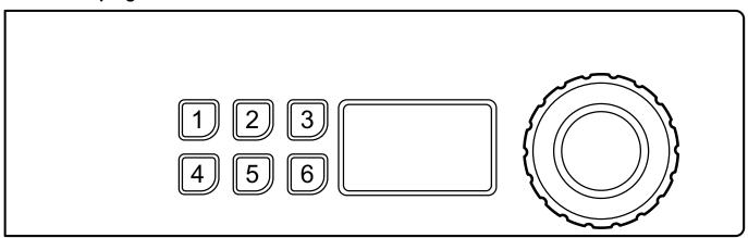
Select program by turning the control knob or select program with the quick selection buttons.
