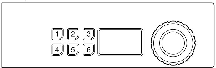
Select program by turning the control knob or select program with the quick selection buttons (if some of the buttons are programmed with this function).
