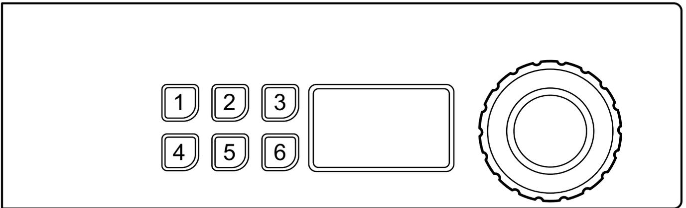
Select program by turning the control knob or select program with the quick selection buttons (if some of the buttons are programmed with this function).
