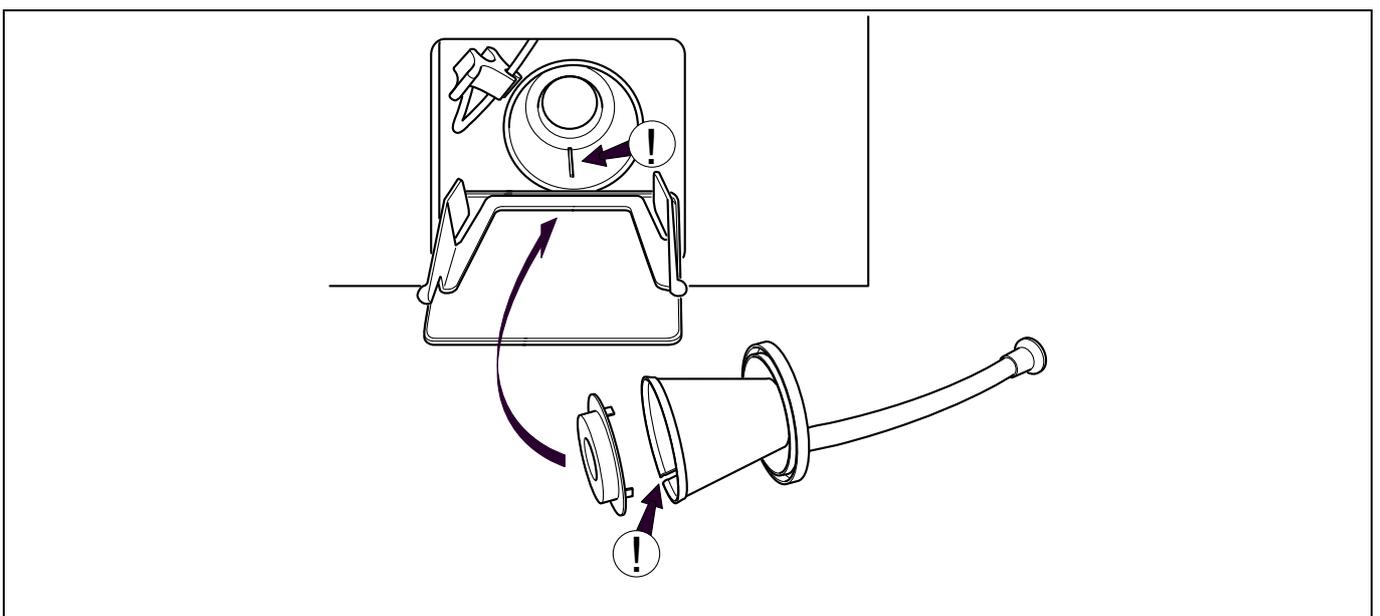
At regular basis, check the drain connection, joints in the drain pipe etc and remove any lint and dust. Clean with for example a small brush. When remounting, make sure the connections are tight.
