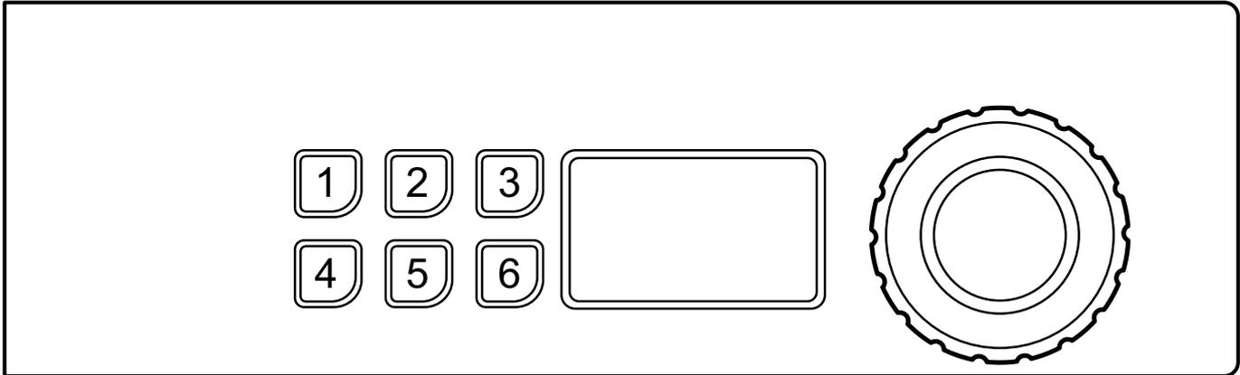
Select program by turning the control knob or select program with the quick selection buttons.
