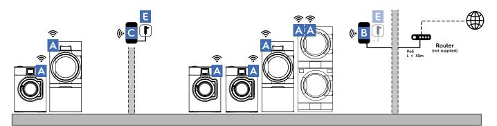
Easy installation Wifi module plugged at the back of the machine.
