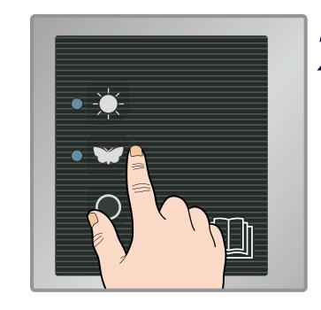
Close the door and press one of the program buttons to start the drying
