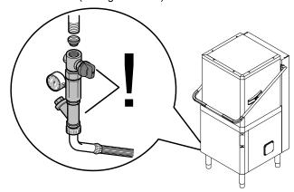
Check that the dynamic water supply pressure, measured between the appliance and the main, is between between 50 and 700 kPa [0.5 - 7 bar] (test while dishwasher tank or boiler is filling with water).
