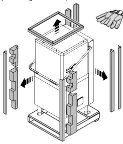
Lift the equipment with a lift truck, remove the base and position it the place of use.
