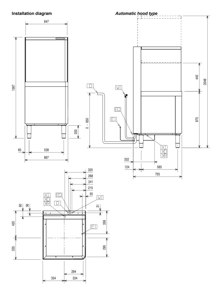
CWI = Cold water Inlet pipe ∅=3/4" G WI = Water Inlet pipe ∅=3/4" G D = Drain pipe internal  $\emptyset$ =40 mm( $\Lambda$ ) - 20 mm( $^*$ )
