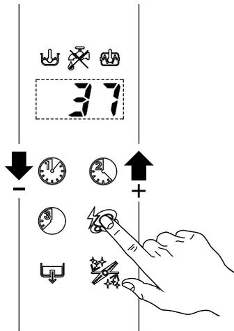
5. to exit the programming mode, press the “Wash cycle 3” button.
