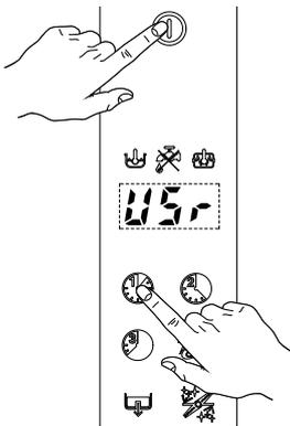
Press the button "L" (refer to F.1 Control panel description) twice to access the detergent and rinse aid adjustment parameters.
