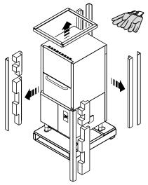
Lift equipment with a lift truck, inserting the forks as indicated below, remove the base and position the appliance where it is to be installed.
