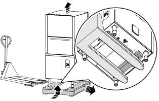
• Remove the wooden spacers "A" on the machine base unscrewing the four "M8" screws.
