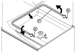
Carefully clean the washing and rinse jets and clean everything with hot water and neutral detergent/detersive, if necessary using a soft brush or sponge. In particular, for the jet "P" use warm water and detergent, and a soft brush "Z" if necessary. Do not use sharp implements to clean the nozzle holes, which could otherwise be damaged.
