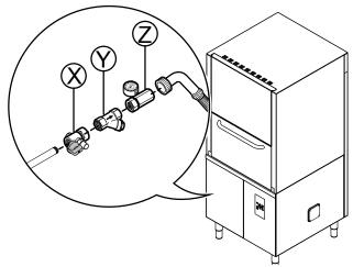
Check that the dynamic water supply pressure, measured between the appliance and the main, is between 50 and 700 kPa [0.5 - 7 bar] (test while dishwasher tank or boiler is filling with water).
