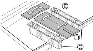
• Clean the filters under a water spray using a nylon brush.
