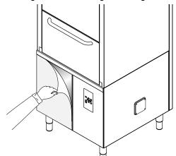
Adjust the equipment by turning the special adjustable feet and making sure it is perfectly level, both length wise and crosswise.
