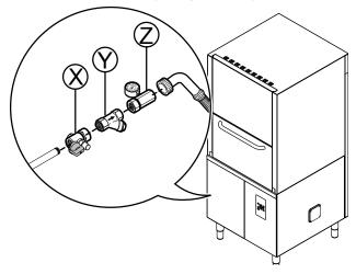
Check that the dynamic water supply pressure, measured between the appliance and the main, is between 50 and 700 kPa [0.5 - 7 bar] (test while dishwasher tank or boiler is filling with water).
