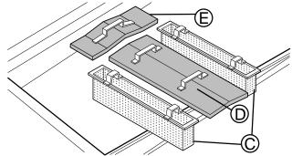
• Clean the filters under a water spray using a nylon brush.
