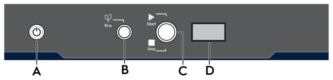
ECO drying button. When the ECO cycle is selected, around the button a green ring is lit up. С Start/Stop button · Press this button to start the drying cycle. Press this button for 5 seconds to stop and
