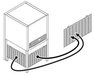
D. Check the air intake filter and remove any objects present.
