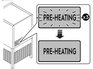
When the equipment reaches the working temperature, the drying cycle starts.
