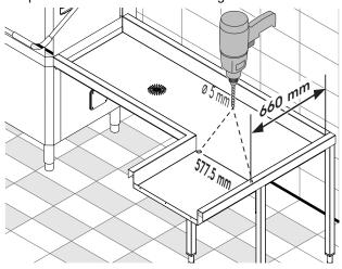
Place the appliance on the table by matching the holes just made with the front feet (see following figure).
