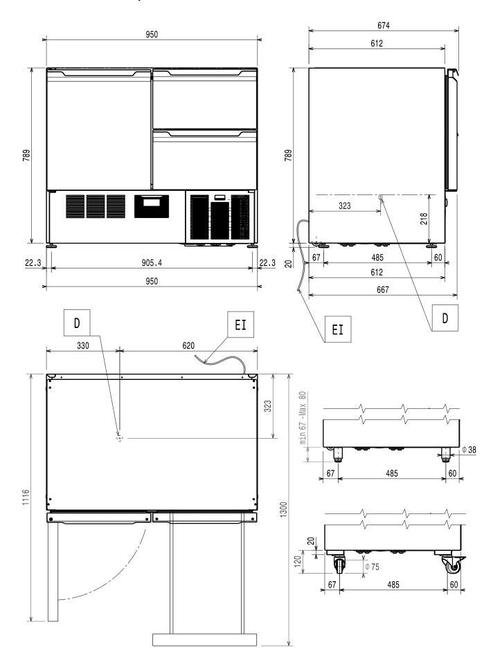
EI = Power cable length TYPE = Certification group SAL95 = Saladette 950 range A = version with chopping-boarding B = version Pizza C = version with steel top D = version without top HC = R290 refrigerant
