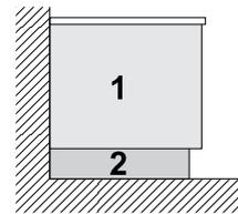
1. Side panels for wall installation: height 400/700/800 mm
