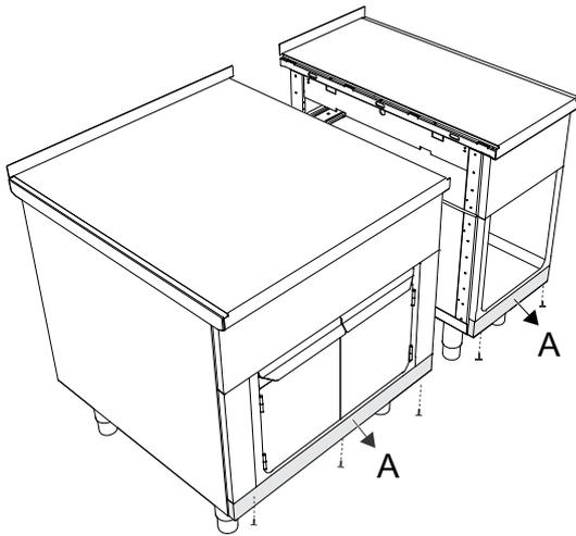
2. Push the units together. Use the adjusting screws on the feet to bring the appliances to the same height, then level them.
