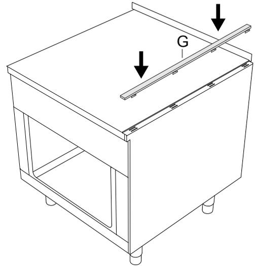
4. Slide end rail **G** in the direction of the arrow to align it to the front.
