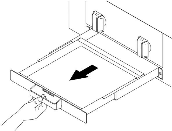
2. Carefully lift the collecting tray out of its fixation. Use both hands to keep it in an horizontal position.
