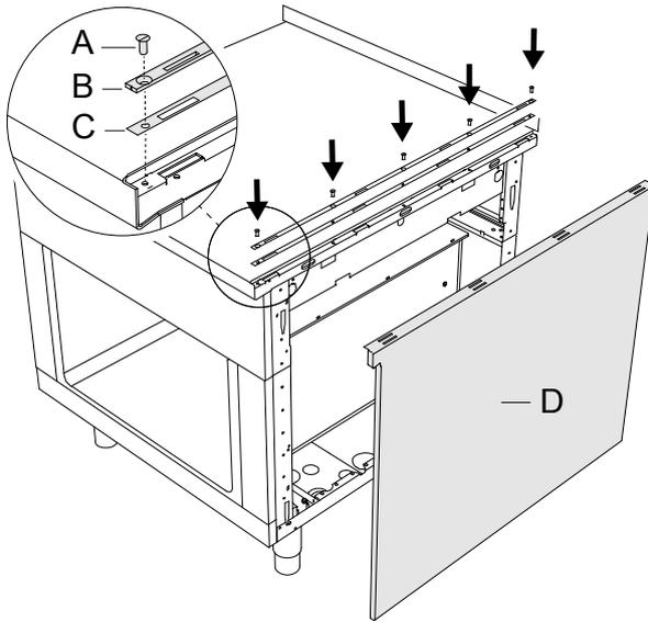
2. Bring the side panel **D** into position. Put the 5 hooks of the panel **F** into the slots **E**.
