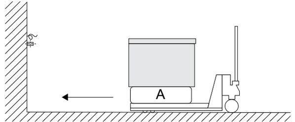
4. Carry the appliance on the lifting cart to the prepared position on the wall and lift it to the correct height.
