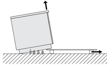
4. Tip the appliance until it is standing on the floor. Then lift at the front and remove the transport pallet.
