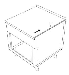
between the appliance and the wall or floor with permanently elastic silicone.
