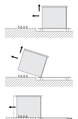
1. Transport the appliance on its transport pallet directly in front of the point of installation.
