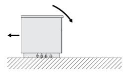
1. Transport the appliance on its pallet to directly in front of the point of installation. The installation connections that are sticking out of the floor should be as close as possible to the side of the transport pallet.
