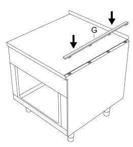
4. Slide end rail **G** in the direction of the arrow to align it to the front.
