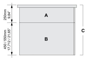
When describing our appliances, we distinguish between top modules A, base modules B and factory-assembled units C. Top and base modules can be set up together or as individual units.
