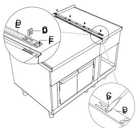
Seal the whole length of the joint with long lasting silicone (we recommend grey junction sealing, code: 059611). Attach the rail D using the supplied screws F. Insert the hook on the underside of cover G into the eyelets in the connecting rail and slide cover G backwards until it aligns to the front.
