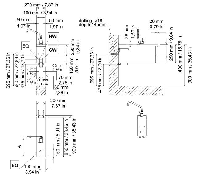
EI = Electrical connection EQ = Potential equalisation HWI = Hot water connection CWI = Cold water connection
