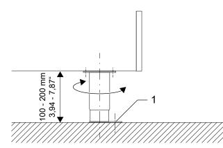
B. Attaching the unit by welding The metal plate underneath the feet must be welded to the floor with a continuous weld around the outer edge.
