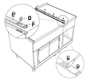
4. Seal the whole length of the joint with long lasting silicone (we recommend grey junction sealing, code: 059611). Attach the rail **D** using the supplied screws **F**. Insert the hook on the underside of cover **G** into the eyelets in the connecting rail and slide cover **G** backwards until it aligns to the front.
