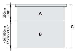
When describing our appliances, we distinguish between top modules A, base modules B and factory-assembled units C. Top and base modules can be set up together or as individual units.
