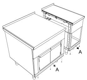
2. Push the units together. Use the adjusting screws on the feet to bring the appliances to the same height, then level them.
