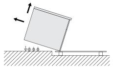
4. Carefully lower the appliance and then move it into the correct position. Finally, remove the transport palette.
