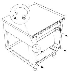
2. Attach connecting rails **C** and **D** with the supplied screws **B**.
