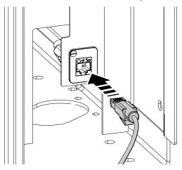
Fig. 1 Ethernet cable into connector
