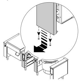
2. Unscrew the bolts and remove the covers.
