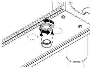
2. Place the Ethernet cable inside the cable gland.
