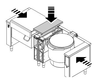
4. Reassemble the user interface panel and the front panel by fixing them with screws.
