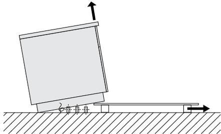
4. Carefully lower the appliance and then move it into the correct position.
