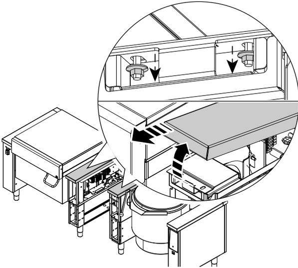
3. Push the units together. Bring the appliances to the same height, then level them. Replace the covers with the double cover required when placing the order, by screwing the bolts.
