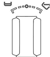
When you release the knob, it returns to the neutral middle position and the appliance remains tilted as it is. To bring it back to the horizontal position, turn the knob counterclockwise (left).
