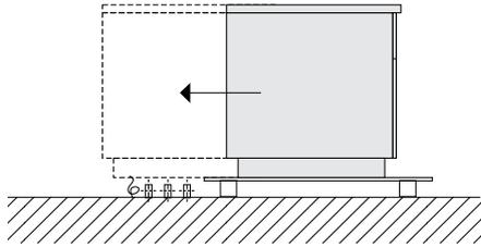
2. Shift the appliance onto the transport pallet such that all of the installation connections lie within the appliance.
