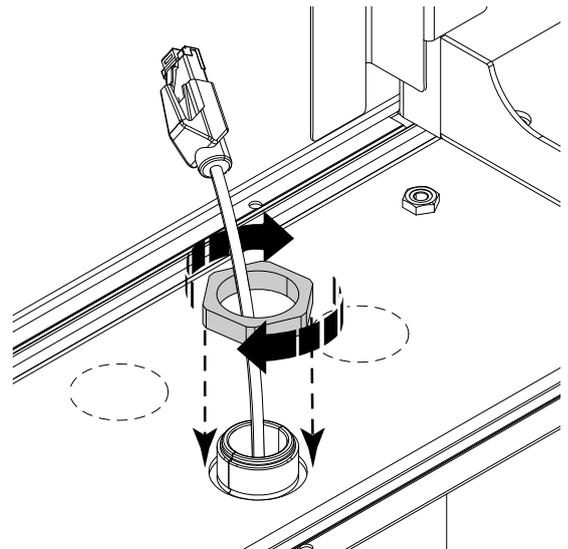
4. Insert the Ethernet cable into the factory-fitted connector, refer to Fig. 1 *Ethernet cable into connector*.
