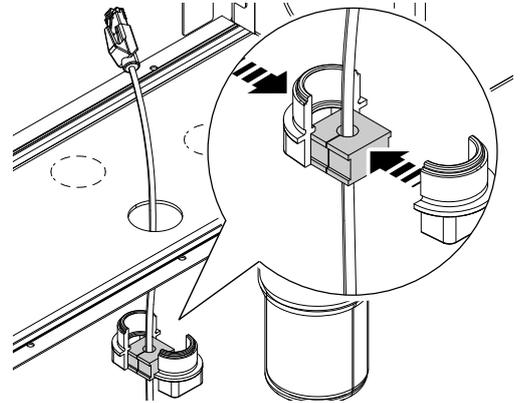
3. Reassemble the cable gland in its original position.
