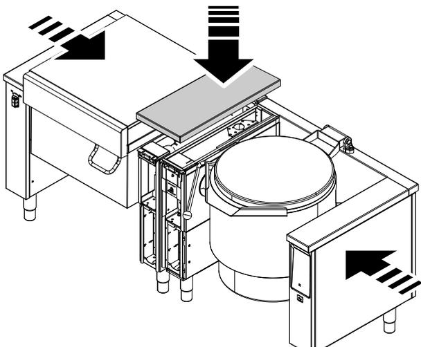
4. Reassemble the user interface panel and the front panel by fixing them with screws.
