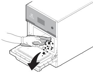
8. Spray the S02 degreaser all inside the cooking cavity and in the inner part of the door.
