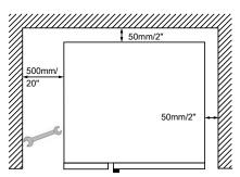
• The left gap must be a minimum of 350 mm if heat sources are acting on the left side of the appliance.
