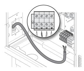
6. After connection secure the cable screwing the cable gland ring.
