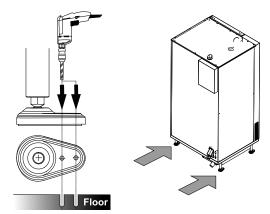
Secure each foot to the floor by means of two appropriate screws that guarantee a minimal force of 0,3 kN.
