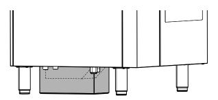
1. The use of the riser is alternative to the cover except for the installations 6 Grids on 10 Grids, where this cover is mandatory.
