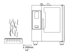
If it is not possible to keep the left side of the appliance a sufficient distance away from heat sources, a heat shield can reduce thermal loads (see accessories catalogue).
