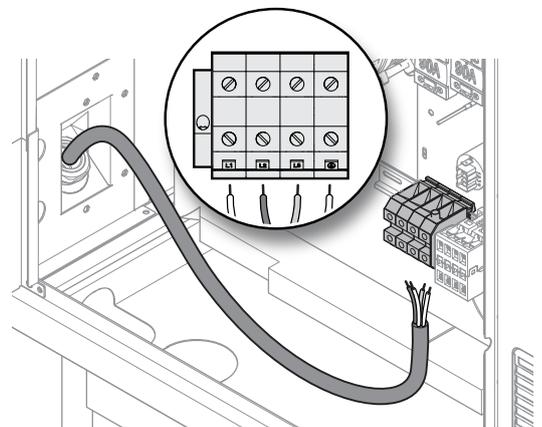
**E.6.2 Power cable installation in electric models**
