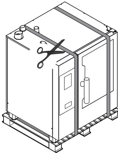
3. Lift the appliance with a lift truck, remove the pallet and position the appliance in the place of use;
