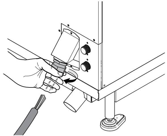
4. Unsheathe all wires from the cable;
