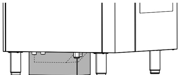
1. The use of the riser is alternative to the cover except for the installations 6 Grids on 10 Grids, where this cover is mandatory.
