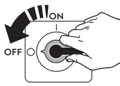
Disconnect the appliance from the power supply before carrying out any installation, assembly, cleaning or maintenance procedure.
