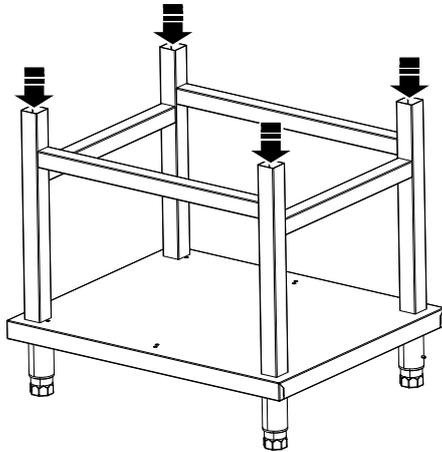
2. Place the appliance onto the oven stand by inserting the locating feet into the tubular uprights.
