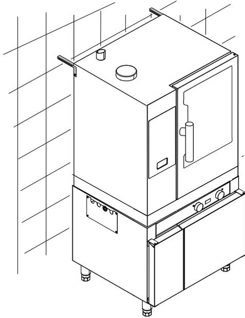
**6 - 10 GN models : Floor fixing with flanged feet**
