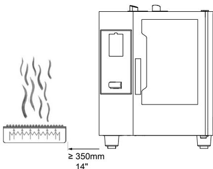
If it is not possible to keep the left side of the appliance a sufficient distance away from heat sources, a heat shield can reduce thermal loads (see accessories catalogue).
