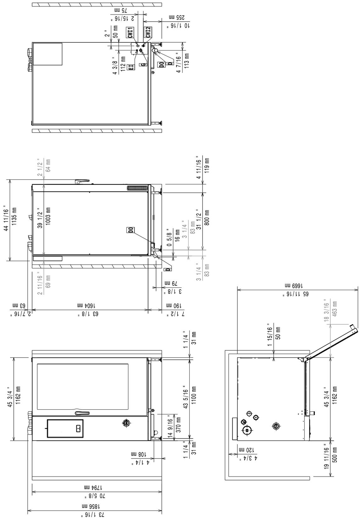
D = Sortie vidange  $\varnothing$ 50 mm M
