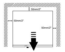
In all models but especially in 20 grids models when possible leave a space of at least 500 mm between the left side of the appliance and the other surfaces to enable maintenance operations.
