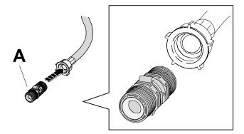
Connect the double check valves A – inserted in the water hoses – to the water taps.
