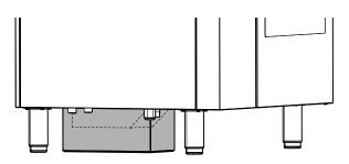
1. The use of the riser is alternative to the cover except for the installations 6 Grids on 10 Grids, where this cover is mandatory.
