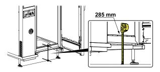
5. After set the front legs of the oven to 285 mm it is necessary to level the oven by correctly adjusting the **rear** legs.
