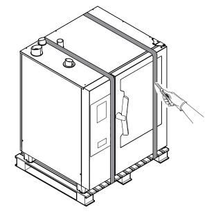
3. Lift the appliance with a lift truck, remove the pallet and position the appliance in the place of use;
