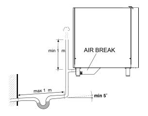
NOTE! An air-break to drain conforms to EN61770 shall be installed before the discharge to the drainage
