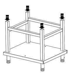
2. Place the appliance onto the oven stand by inserting the locating feet into the tubular uprights.
