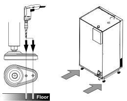
Secure each foot to the floor by means of two appropriate screws that guarantee a minimal force of 0,3 kN.
