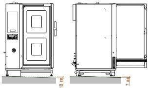
2. In case the floor slope is above the limits, "Leveling ramp" is mandatory.
