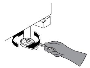
4. Measure it from the cavity to the floor. The measurement should be taken in the centre, then check that left side and right side must be within the tolerance of  $\pm$  2.5 mm. See the illustration below.
