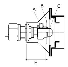
figure A - Burner injector
