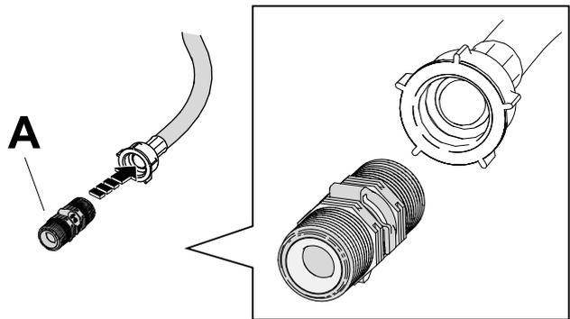
3. Connect the double check valves A – inserted in the water hoses – to the water taps.
