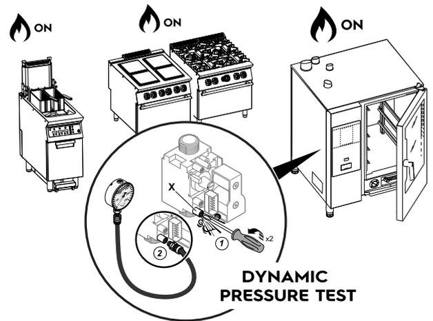
1. Remove the left hand side panel to gain access to the gas valve;
