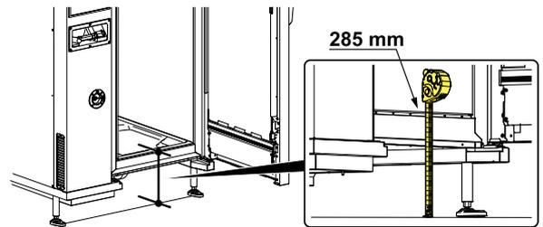
5. After set the front legs of the oven to 285 mm it is necessary to level the oven by correctly adjusting the **rear** legs.
