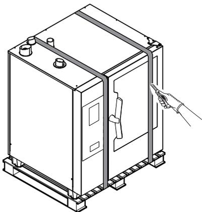
3. Lift the appliance with a lift truck, remove the pallet and position the appliance in the place of use;
