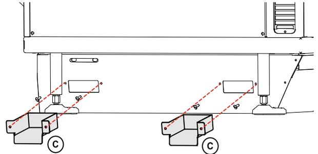
Once the watertight assembly has been done in accordance with the above procedure, it will prevent liquid spillage on adjacent floor surface from passing under inaccessible portions of the appliance.
