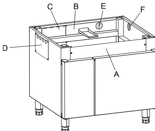
2. Replace the oven feet with the special feet supplied with the cupboard accessory;
