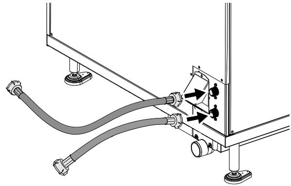
2. Insert the double check valves A – supplied with the appliance – into the other end of the water hoses. Make sure they are inserted in the correct position and direction.
