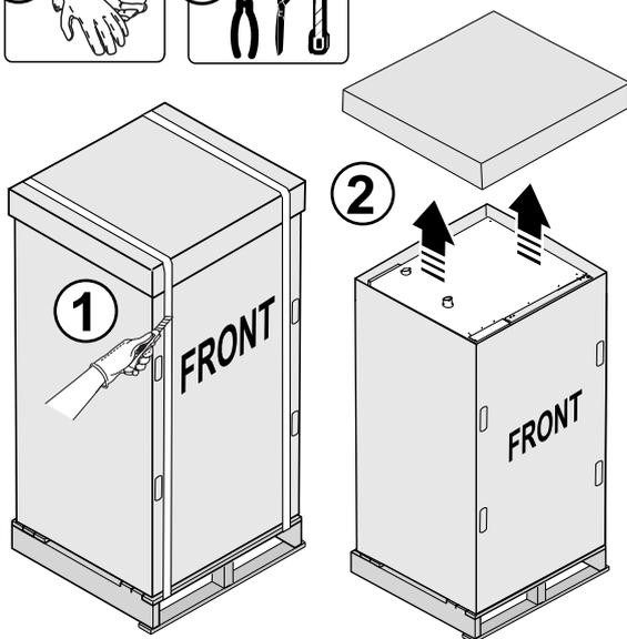
3. Remove the upper cardboard corners, the protection for the handle and the 4 cardboard wrapping the appliance;
