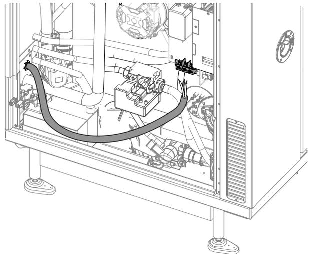
6. After connection secure the cable screwing the cable gland ring.
