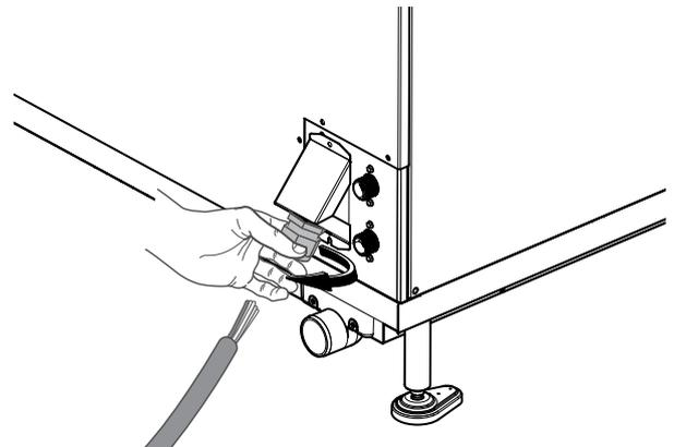
4. Unsheathe all wires from the cable;
