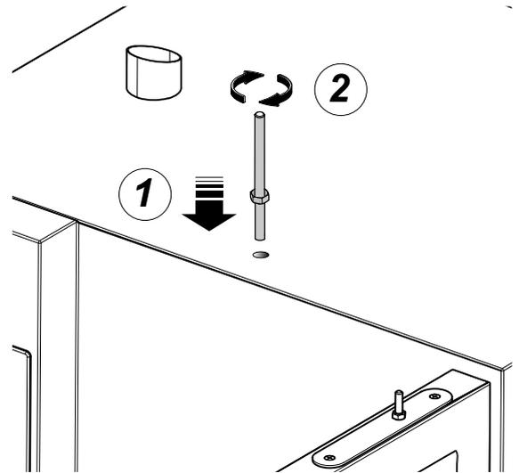
3. Mount all elements - from 2 to 9 – on the top panel of the oven as shown in the figure.
