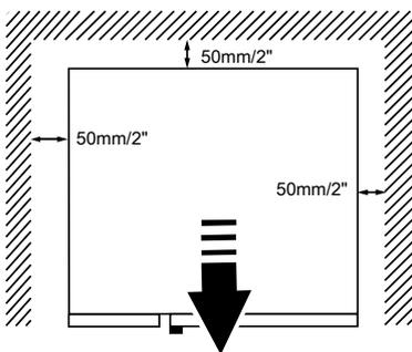
In all models but especially in 20 grids models when possible leave a space of at least 500 mm between the left side of the appliance and the other surfaces to enable maintenance operations.
