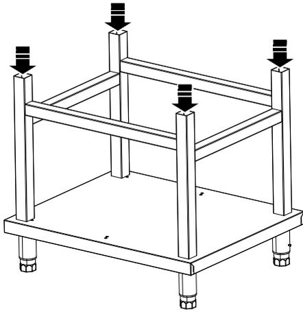
2. Using appropriate lifting equipment, position the appliance on the oven stand by inserting the locating feet into the tubular uprights.
