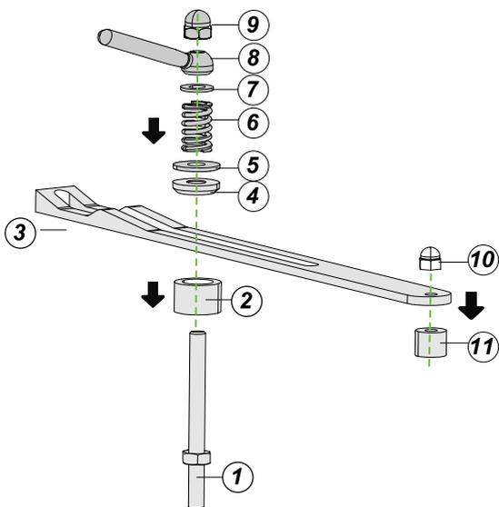
2. Insert the pin – element 1 - into the hole on the oven top panel. Screw the pin in until it locks. See the following figure.
