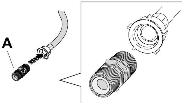
3. Connect the double check valves A – inserted in the water hoses – to the water taps.
