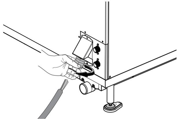
4. Unsheathe all wires from the cable;
