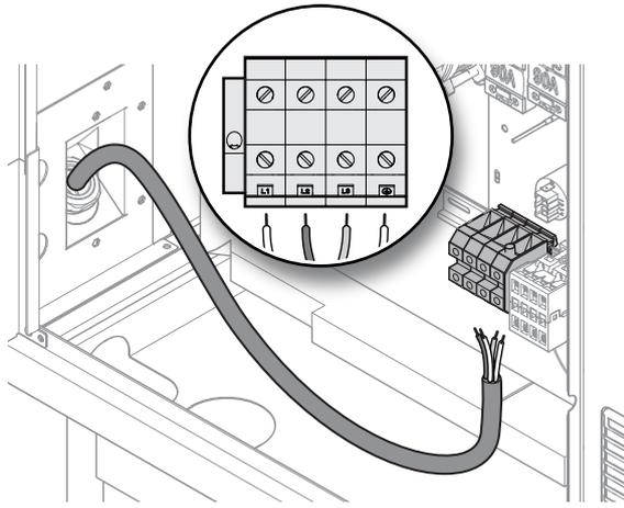
7. After connection secure the cable screwing the cable gland ring.
