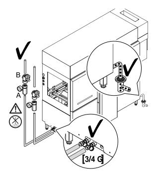
Fig. 3 Plumbing connection for left machine
