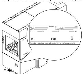
Fig. 1 Data plate position (machine right)
