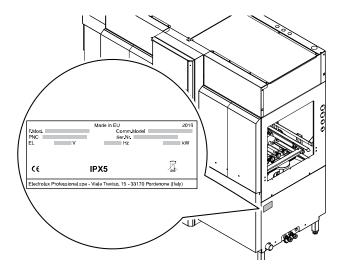
Fig. 2 Data plate position (machine left)
