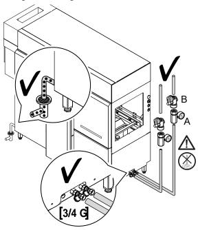
Fig. 4 Plumbing connection for right machine
