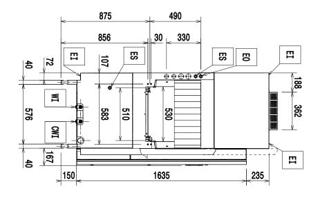
Installation diagram 150 racks/hour left to right
