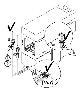
Fig. 3 Plumbing connection for left machine
