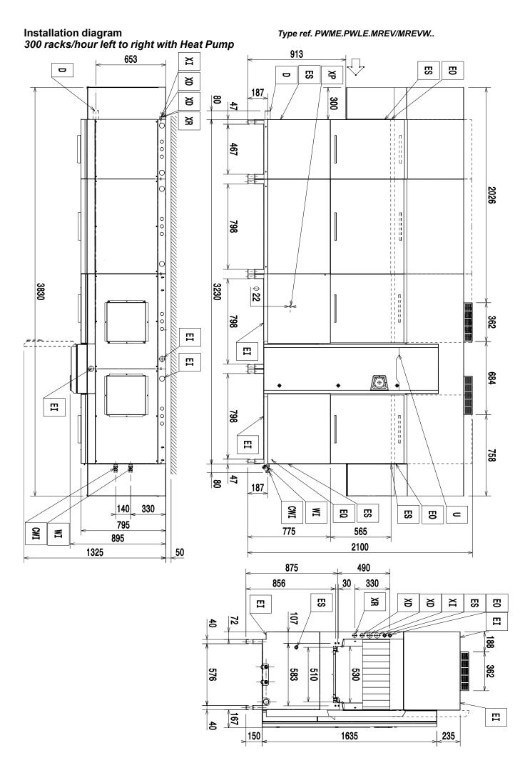
D = Drain outlet ⊘=50mm (external) EI = Electricity inlet EO = Electricity outlet ES = Electrical signal IN/OUT EQ = Equipotential screw XD= Pipe inlet for detergent XR= Pipe inlet for rinse-aid XI= Pipe inlet for delime XP= Chemicals probe/sensor WI = Water inlet G 3/4" CWI = Cold water inlet G 3/4" U = USB V = Vent(s)
