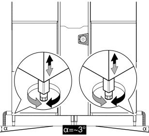
Adjust the machine crosswise with a minimum inclination of 3° in order to facilitate the drainage of the dirty water from the tanks.
