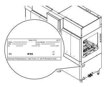
Fig. 2 Data plate position (machine left)
