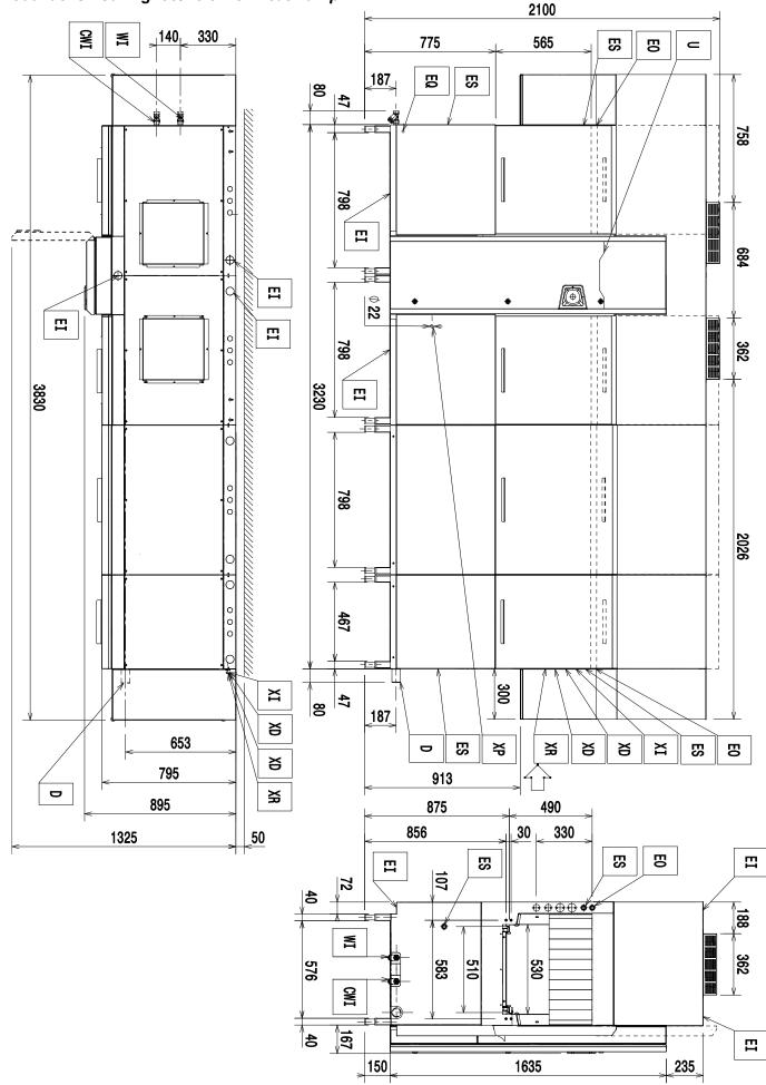
Installation diagram 300 racks/hour left to right
