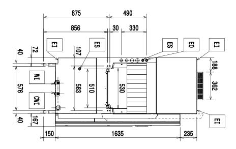
Installation diagram 200 racks/hour left to right
