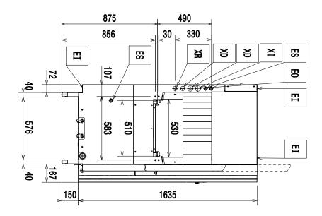
Installation diagram 200 racks/hour left to right with Heat Pump
