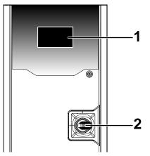
1 Touch screen with direct selection of functions. Touch the selected icons to activate the corresponding functions.
