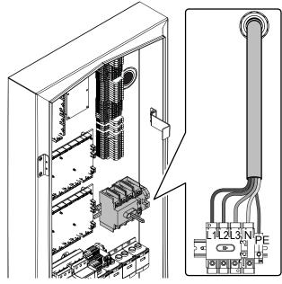
activate all the contactors by turning clockwise the contactor knob from position "O" to "I";
