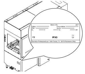
Fig. 1 Data plate position (machine right)
