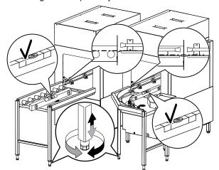
Refer to the instruction provided with the rack handling system to complete the installation.  Apply silicone¹ "C" between the dishwasher and the rack handling system.
