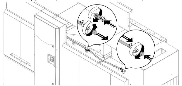
17. Replace the default heating element of the machine boiler with the new one provided with the kit.
