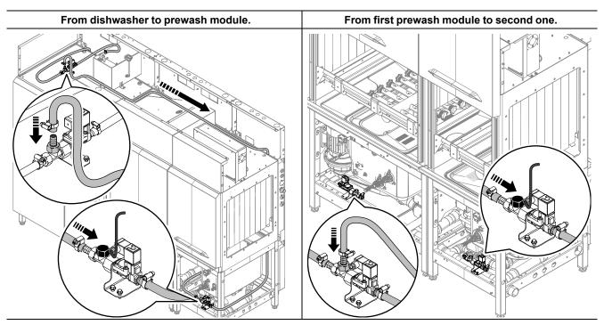
15. Connect the door cleaning system of the prewash module. Do the same to connect the second prewash.
