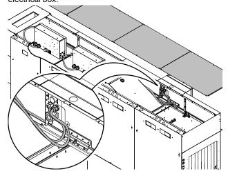
Pass the wiring cables through the cable gland "A" and connect the power cables "L1", "L2" and "L3" to the terminal board as shown in the picture. Insert the yellow/green ground cable together with those already present.
