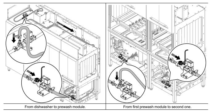
16. Connect the door cleaning system of the prewash module. Do the same to connect the second prewash.
