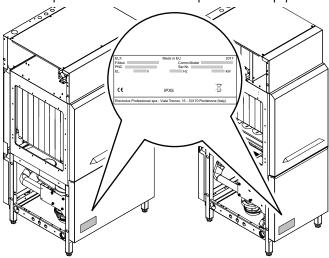
Fig. 1 Data plate position
