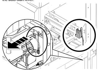
3. Refit the lever and its sensor into the prewash module or in the second prewash module.
