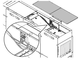
Pass the wiring cables through the cable gland "A" and connect the power cables "L1", "L2" and "L3" to the terminal board as shown in the picture. Insert the yellow/green ground cable together with those already present.
