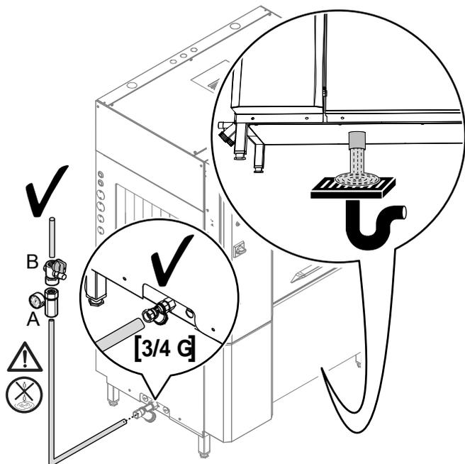
Fig. 2 Raccordement hydraulique
