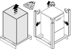
• Lift the equipment with a lift truck, remove the base and position it the place of use.
