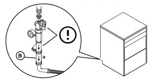
Check that the dynamic water supply pressure, measured between the appliance and the main, is between 1.8 bar [180 kPa] and 3 bar [300 kPa] for machines with pressure boiler and between 0.5 bar [50 kPa] and 7 bar [700 kPa] for machines with atmospheric boiler (test while dishwasher tank or boiler is filling with water).
