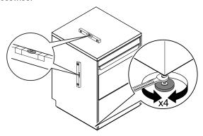
If the dishwasher is installed under a work plan, the dimensions of the space, where it is inserted, must be the same as those shown in the following figure. Position the dishwasher and level the appliance by turning the relative height-adjustable feet.
