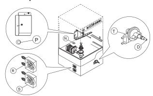
There is a ready-made impression "N" to be perforated ( $\varnothing$  8 mm) for positioning the detergent concentration measuring sensor.
