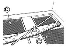
Make sure the upper and lower wash and rinse arms are correctly fitted.
