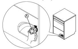
• Pour approx. 1.5 kg of coarse salt [NaCl] in container "A" (an amount sufficient to fill the salt container up to the rim) using the special funnel supplied (see figure below).
