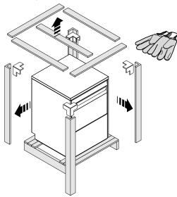
Lift the equipment with a lift truck, remove the base and position it the place of use.
