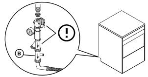
Check that the dynamic water supply pressure, measured between the appliance and the main, is between 2 bar [200 kPa] and 3 bar [300 kPa] for machines with pressure boiler and between 0.5 bar [50 kPa] and 7 bar [700 kPa] for machines with atmospheric boiler (test while dishwasher tank or boiler is filling with water).
