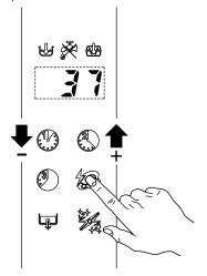
to exit the programming mode, press the "Wash cycle 3" button.
