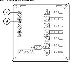
Connect the rinse-aid dispenser between terminals 8 and 9. These connection points are live during filling of the tank and at the end of the rinse cycle for a set time (see H.2 Setting the dispensers paragraph).
