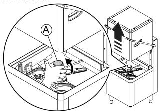
Pour approx. 2 kg of coarse salt [NaCl] in container "A" (an amount sufficient to fill the salt container up to the rim) using the special funnel supplied.
