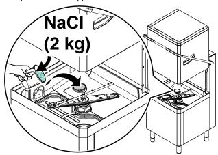
Remove any traces of salt from the filling hole and the container thread of the closing cap.
