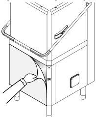
Adjust the equipment by turning the special adjustable feet and making sure it is perfectly level, both length wise and crosswise.
