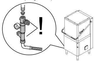
Check that the dynamic water supply pressure, measured between the appliance and the main, is between between 50 and 700 kPa [0.5 - 7 bar] (test while dishwasher tank or boiler is filling with water).
