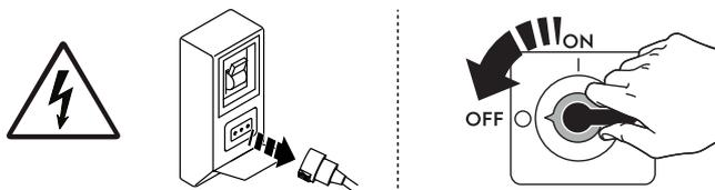
Disconnect the appliance from the power supply before carrying out any installation, assembly, cleaning or maintenance procedure.
