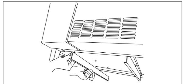
7. Take the tray located inside the compartment and slide it onto the support guides.
