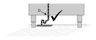
The drain diameter is  $1\frac{1}{2}$ ", therefore it is advisable to use a  $1\frac{1}{2}$ " drain pipe or to a diameter 25 mm hose.
