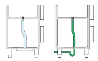
The drain diameter is  $1\frac{1}{2}$ ", therefore it is advisable to use a  $1\frac{1}{2}$ " drain pipe.
