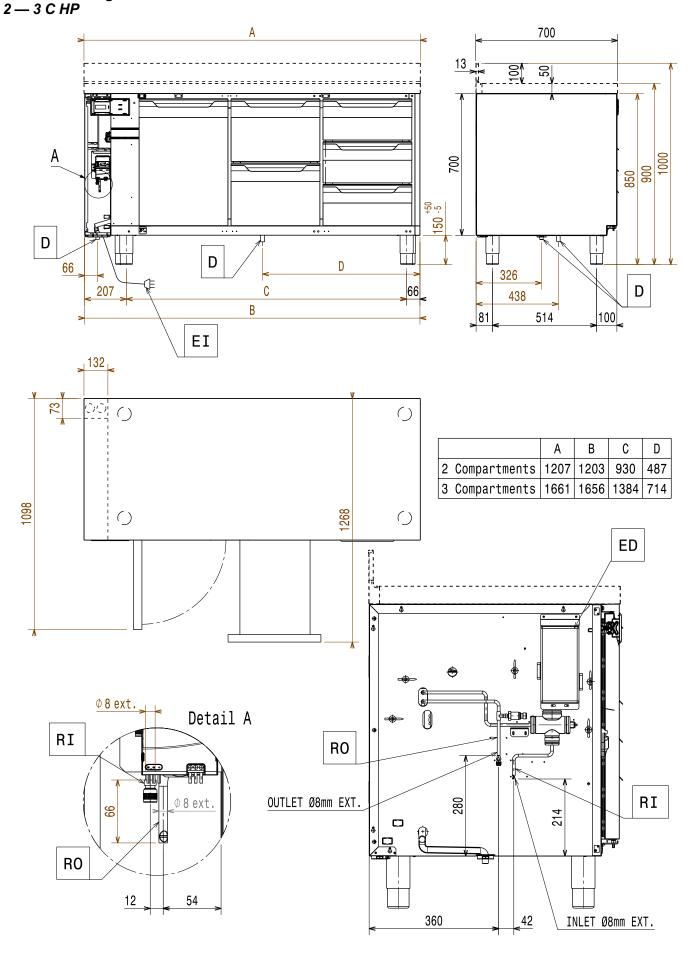
EI = Power cable length ED = Electrical connections D = Compartment drain hole RI = Refrigerant inlet (liquid) RO = Refrigerant outlet (gas)
