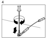
The cable must then be fixed to the wall with a plug, to permanently secure the appliance;
