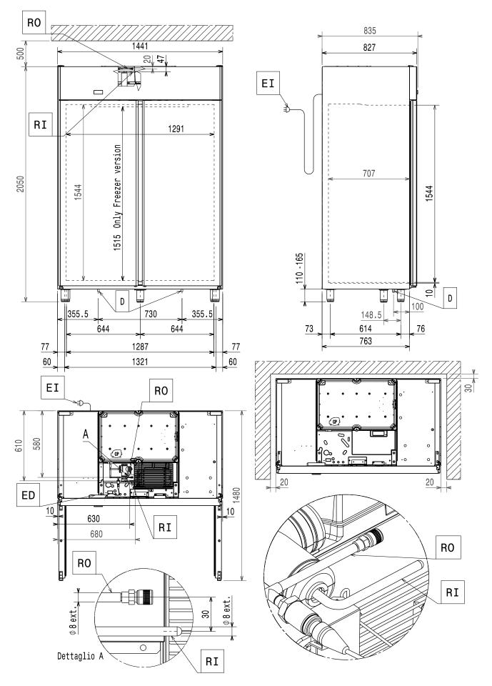
Model with 1 door – CO2 remote unit without valve
