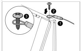
4. retighten the screw complete with the cable on the roof of the appliance;
