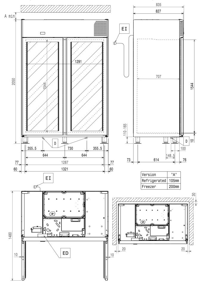
ED = Electrical connections EI = Power cable length D = Compartment drain hole RI = Refrigerant Inlet (liquid) RO = Refrigerant Outlet (gas)
