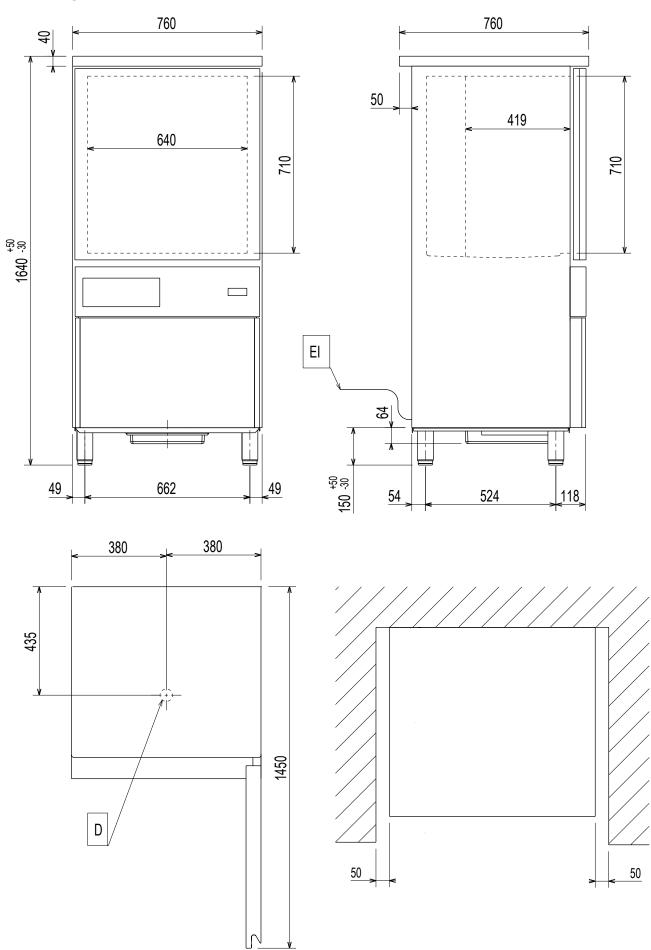
Installation diagram model 28kg GN 1/1 remote
