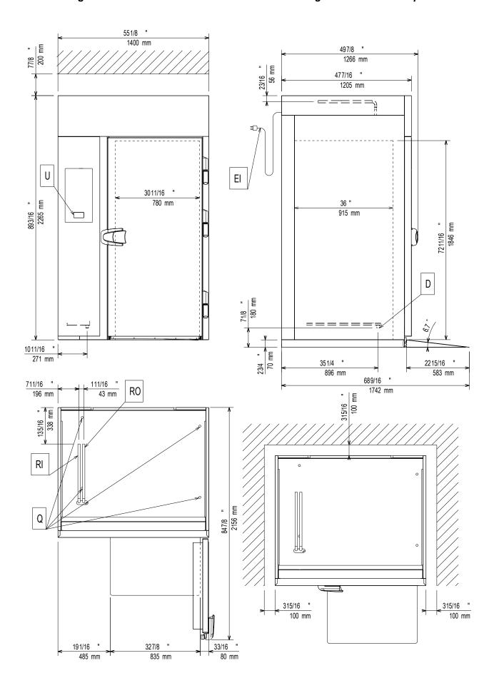
EI = Power cable length WIC = Cooling water inlet WOC = Cooling water outlet RI = Refrigerant inlet (liquid) RO = Refrigerant outlet (gas)
