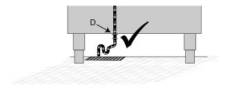
For 6GN 1/1 — 10GN 1/1 — 10GN 2/1 models , the drain diameter is  $1\frac{1}{2}$ ", therefore it is advisable to use a  $1\frac{1}{2}$ " drain pipe or to a diameter 25mm hose.
