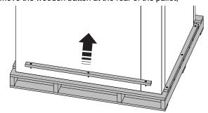
slide the equipment in, taking care not to damage the bottom;
