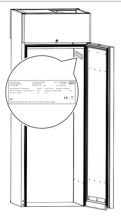
Fig. 1 Marking plate position
