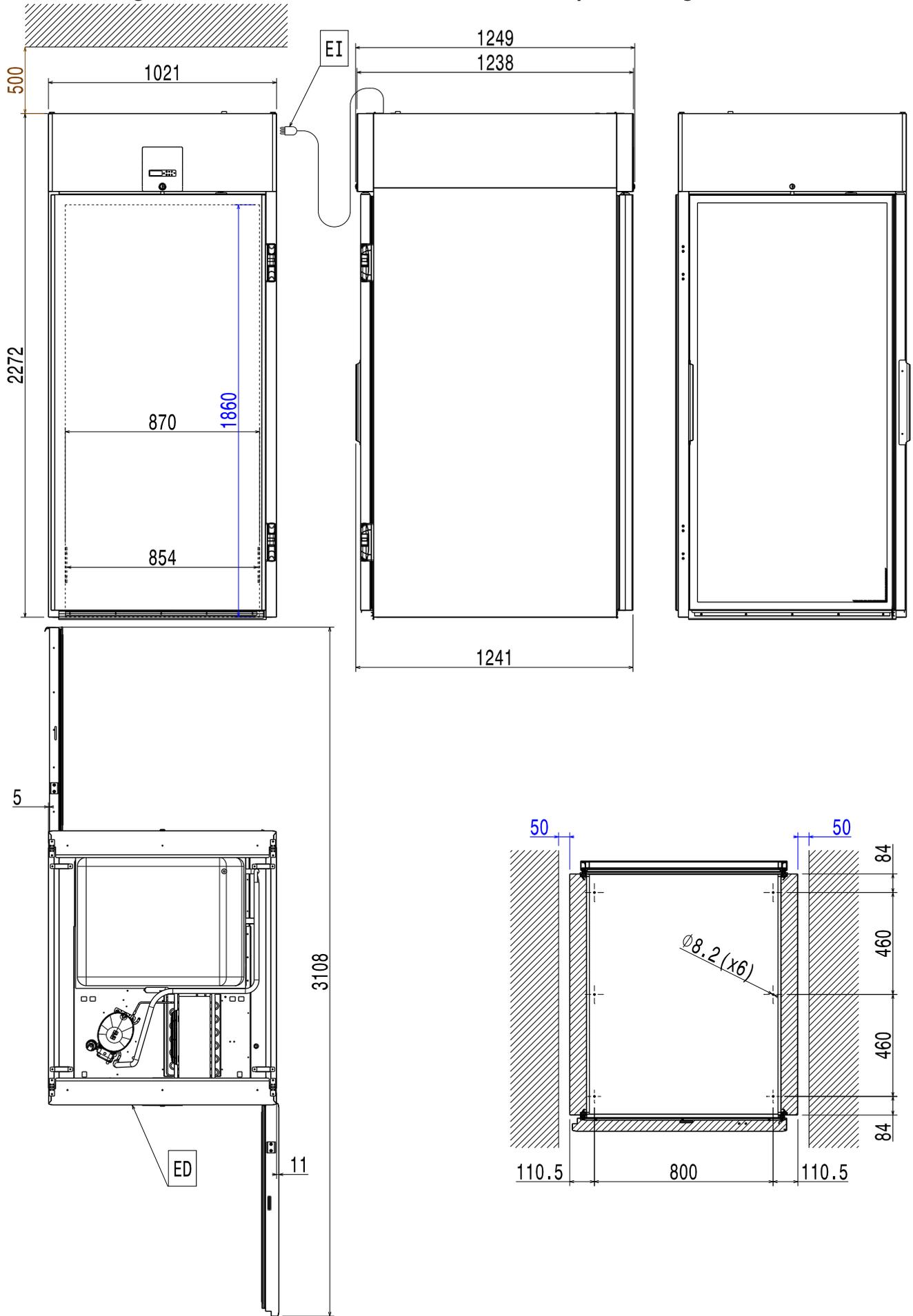
EI = Power cable length 3500 mm, Schuko socket
